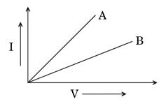
Two metallic resistors are connected first in series and then in parallel across a d.c. supply. Plot of I-V graph is shown for the two cases. Which one represents a parallel combination of the resistors and why?
